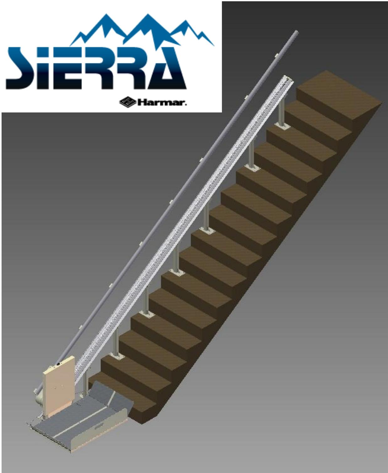
Position track mounting legs on steps. The number of legs and spacing will be determined by the overall length and number of pieces of track. If your lift was ordered with the track pre-cut to length, a drawing for your specific installation will detail the leg locations.
