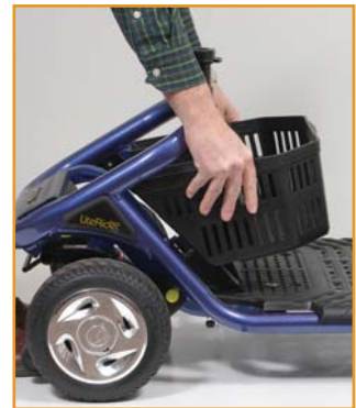
Remove the baskets from under the seat and from the tiller (not shown)
