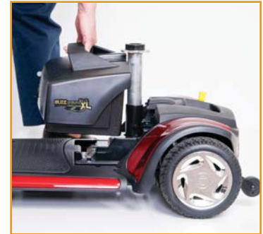
Step 2: Pull out the battery pack!
