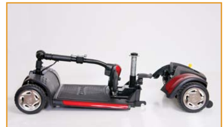
Step 3: Pull up on the drivetrain release lever to separate the front and rear frame sections!
