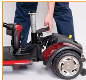
Step 3: Pull up on the drivetrain release lever to separate the front and rear frame sections!
