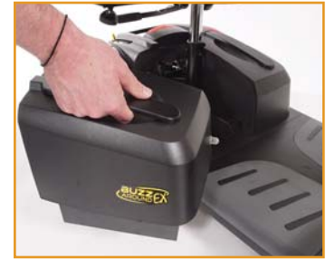
Step 2: Pull out the battery pack!
