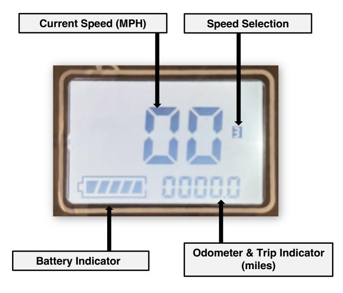
The odometer (total miles ridden) will display for approximately 5 seconds when then scooter is turned on. After approximately 5 seconds, the trip indicator will display for the rest of the time the scooter is turned on.
