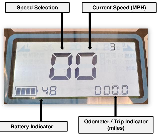
A full charge of the battery will be 55-56 volts. It may take 5-10 discharge are recharge cycles before the batteries break in fully and allow the total charge to reach 55-56 volts.
