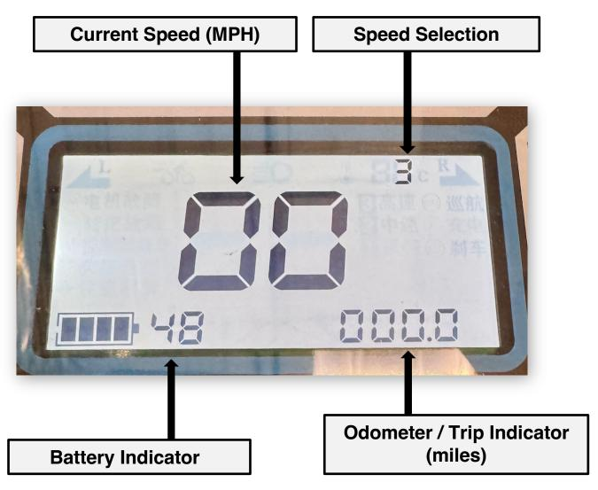
A full charge of the battery will be 55-56 volts. It may take 5-10 discharge are recharge cycles before the batteries break in fully and allow the total charge to reach 55-56 volts.
