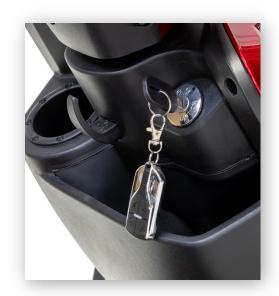
The key fob has four buttons. One to arm the alarm system, one to disarm the alarm
