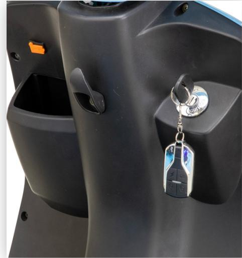
The key fob has four buttons. One to arm the alarm system, one to disarm the alarm system, one to remotely start the scooter, and one that acts as a “panic” button which sounds the alarm.
