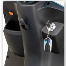
The key fob has four buttons. One to arm the alarm system, one to disarm the alarm system, one to remotely start the scooter, and one that acts as a "panic" button which sounds the alarm.
