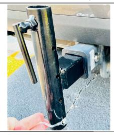
Install the ①Hitch Adapter into the hitch of vehicle.
