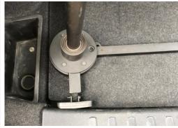
Ratchet the Welter frame against the rear seat and boot lip by pushing the ratchet lever up and down until the frame is fully secured.
