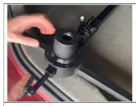
Screw in the Boom leg on the securing bar and using the ratchet lever.
