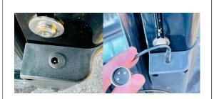
On the side of the motor on your Welterweight Power Boom, there is a Port for the Power Cord. Plug The Power Cord into the optional Battery Pack – or – Plug the Power Cord directly into the Joystick of thefold-ablewheelchair or the Charging Port on mobility Scooter.
