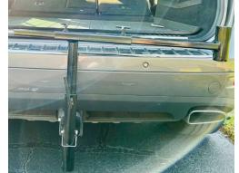
Fits the ③Boom Receiving Plate into the ② Swivel Bar, which is adjustable for your best and preferred lifting angle.
