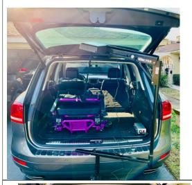
Use the Remote, or The Raise/Lower Switch on the Boom to lift the Scooter or Wheelchair into your trunk.
