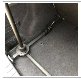
Next is attaching The Power Boom on the Boom base and unfold the Power Boom.
