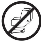
Ball Mount Hitch Adapter can NOT be used when installing a Swing Away
