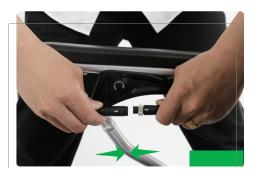
6.Connect the controller wireharnessto the CPU wireharness.
