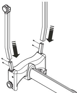
3. Using Allen Key provided, tighten the 6mm screws located on each side of the chassis.
