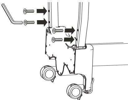
4. Insert the curved boom section into the boom carriage. Secure the assembly by inserting the two 6mm countersunk screws into the blue capping plate provided in the fastener kit, as shown below and tighten firmly.
