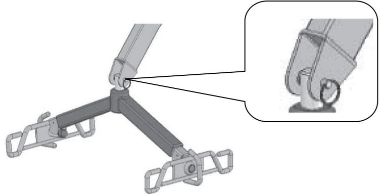
11. Attach the spreader bar bracket to the boom and insert retainer pin. Insert Retaining ring through retainer pin to secure spreader bar to boom.
