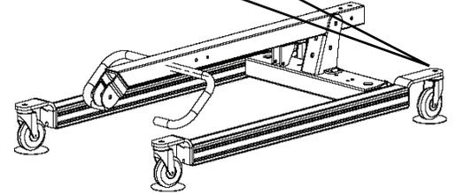
2. Remove the bolts from the bottom of the mast and base.
