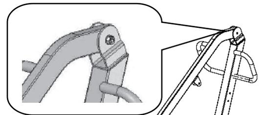
6. Reinstall the bolts in the holes at bottom of mast. Tighten the nuts.
