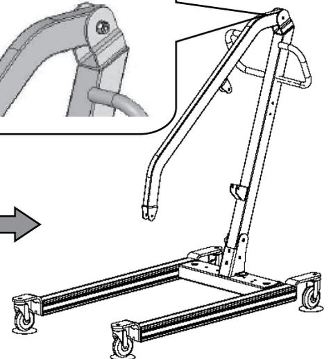
7. Attach the control box hanging bracket to the mast. Tighten the nuts.
