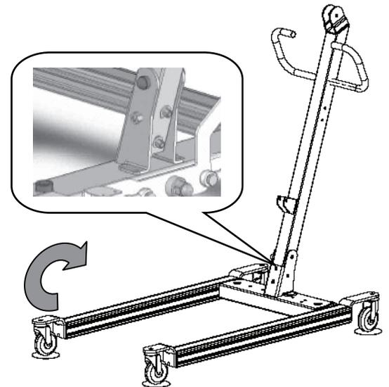
4. Reinstall the bolts in the holes at bottom of mast. Tighten the nuts.
