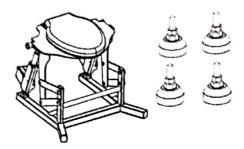
Lift the 4 feet of the bottom frame of the toilet seat in turn, and align the feet with the screw holes at the bottom.
