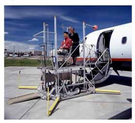
The Mobilift AX / AXR is used to enplane and deplane disabled passengers on regional and narrow body aircraft that are ground loading. The lifts comply with the US Air Carrier Access Act requirements and the FAA regulations for boarding lifts. The lift protects both the passenger and the airline employee from the risks of hand carrying a boarding chair.
