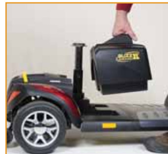
Step 2: Pull out the battery pack!
