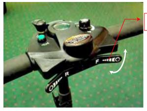
Finger Lever Control/Maximum Force Applied on Lever is 4N
