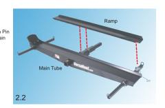
Slide the Ramp Double Tab Bracket over the Main Tube, and secure with the ¼" x ¾" Bolts. Slide the Ramp Lock Bracket over the Tie Down Tube. Do NOT over tighten (Figure 2.1). Slide the Ramp onto the Lock Bracket tabs. Lock the Lynch Pin into place (Figure 2.2).
