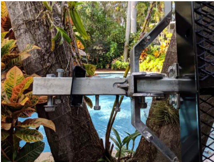
Class III Hitch Ready With Noise / Vibration Reduction plate, ready to be attached to your vehicle.
