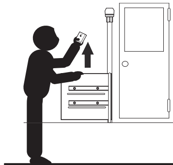
5. Raise platform till it latches securely.
