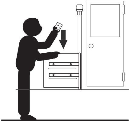
1. Remove Safety pin and lower plate.
