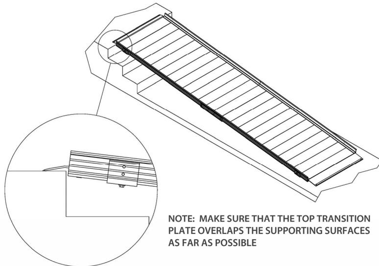
3.6. **ANCHOR RAMP UPPER TRANSITION:** The MRUT (RAMP UPPER TRANSITION) must be anchored to a substantial surface. Use the pre-drilled holes at each corner of the upper transition as guides.
