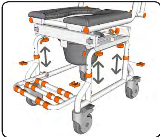
To adjust the seat height remove the securing clips and slide the height adjustment tubes up or down to the required height.
