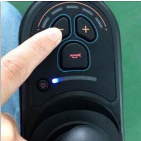
4) Saving Parameter setting: After choosing proper parameter, long press “+” & “-” buttons for 3 seconds, save and quit, return to run.
