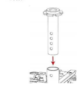
From behind the product, looking forward, insert the seat bolt into hole on the left side of the seat post. This bolt is also used to adjust the seat height. Insert the bolt as far into the hole as it will go, making sure that the bolt passes all the way through to the hole on the opposite side. Install the washer and nut and tighten them using the included flat wrench.
