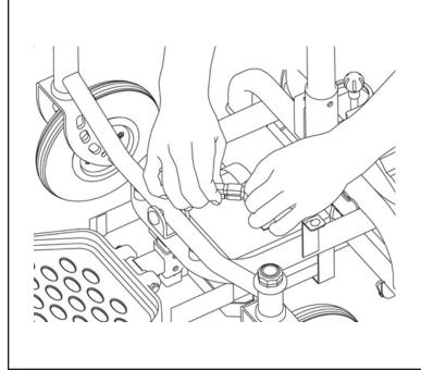
**6** Replace the cover shroud. Replace and tighten the two knobs removed in Step 1.
