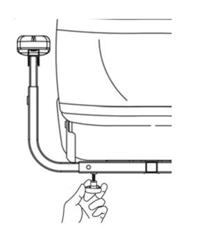
Insert the controller's square tube into the tube under the armrest. Tighten the bolt on the underside of the controller arm tube to hold it in place at the desired extension.
