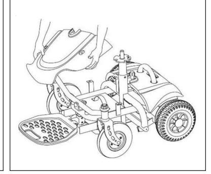
Lift the seat and pull the swivel lever up at the same time. Lower the bottom of the seat onto the seat post. Release the lever, swivel the seat and push down on the seat until it locks in place.
