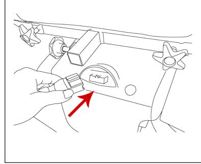
Fully charge the wheelchair's batteries by inserting the round charger connector into the battery charging terminal on the front of the wheelchair's controller and inserting the 3-pronged plug into a standard electrical outlet.
