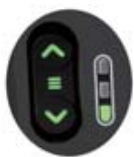
Figure 38: Drive function select button and display
