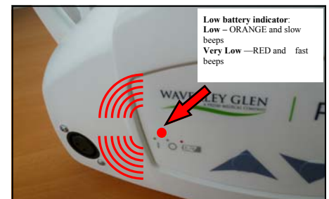
Figure 4D - If the indicator light is ORANGE or RED in color then the batteries of the lift are low and should be charged.
