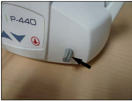
Figure 15A - Gray rubber grommet located on front left side of the lift. Rubber airline is not connected. Note ridge on grommet.
