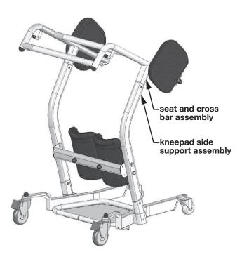
6. Insert the seat and cross bar assembly into the tubes at the top of the kneepad side support assembly as shown above.
