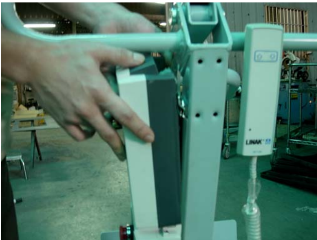
Fit battery onto control box.
