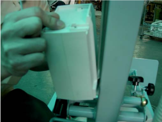
Fit control box onto bracket (on mast).
